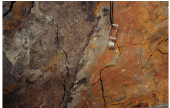
Photo 1 – West looking view of the south dipping fault in the trench. Note knife-edge contact and contorted zones on either side.
