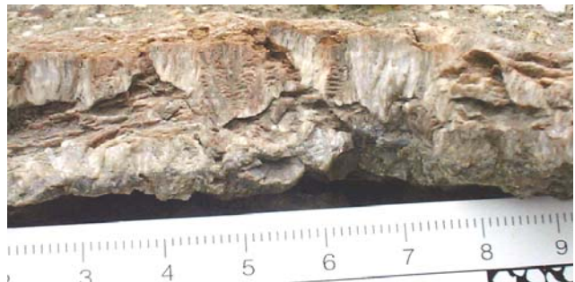
Cross section through disk showing the fibrous nature of the calcitic material and the cone in cone structures.
